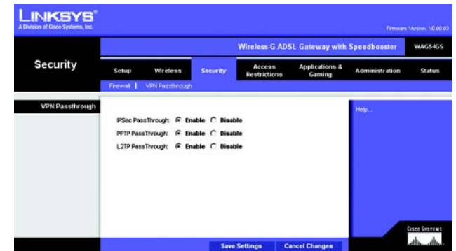
Figure 6-25 : VPN Passthrough (Intercommunication VPN)
